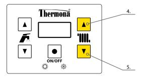
Shift the equithermic curve using buttons 4 and 5.
